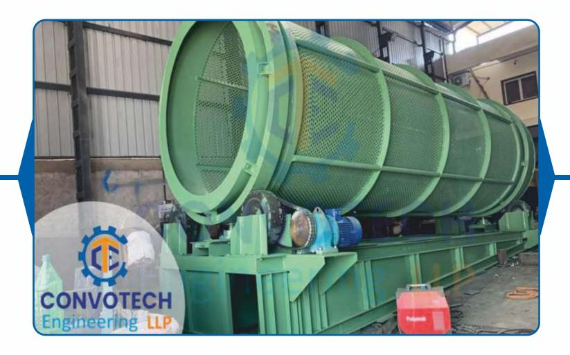
The Goal of **Convotech Engineering LLP** is to help you convert this waste into recycled waste and aggregation which has a range of uses in various construction applications. **Convotech Engineering LLP** manufacturer scientifically designed Trommel Screen. Trommel Screen effectively composts based on properties of particle size and density.
